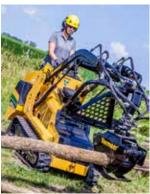
The universal attachment plate allows for quick change of attachments. A dual auxiliary circuit option on the auxiliary hydraulic system is available for attachments that require highflow/low-flow circuits
